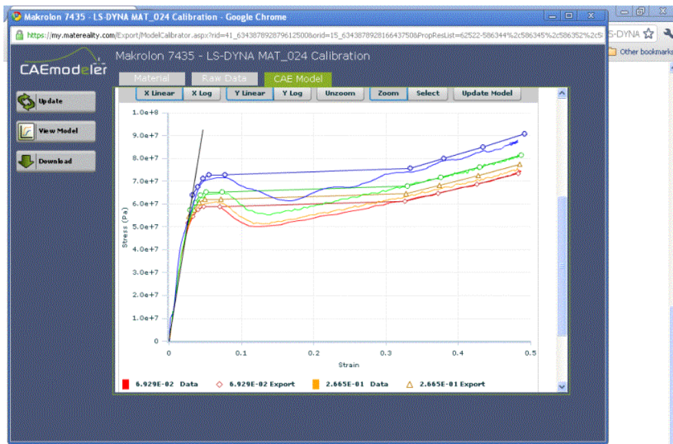
Figure 6 Finalized material model viewed against raw tensile test data
