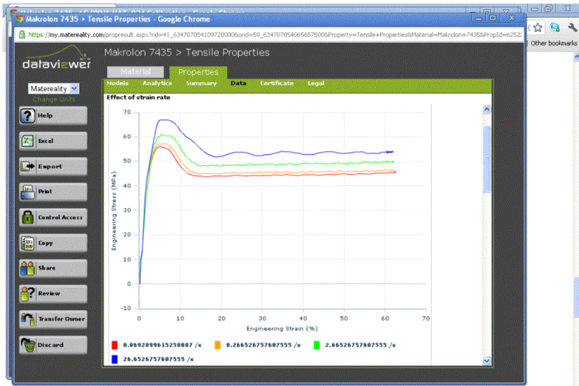
Figure 1 Typical rate-dependent tensile data for a plastic
